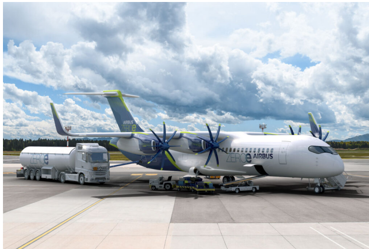
Figure 31 : Hydrogen refueling through a hydrogen truck
